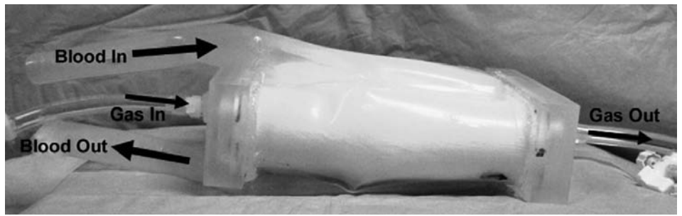
Abb. 6: Compliant Thoracic Artificial Lung (cTAL) [20]
